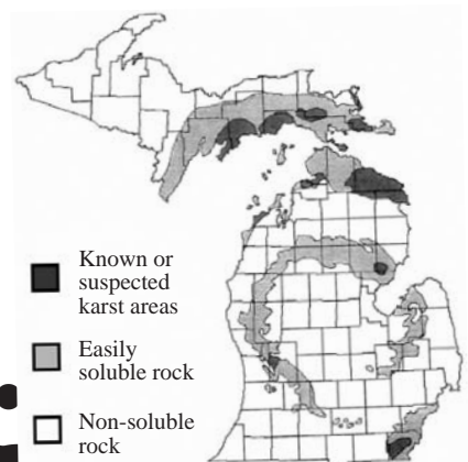
Figure 3: Bedrock areas of concern. “Understanding Groundwater.” Institute of Water Research/Center for Remote Sensing, MSU.
